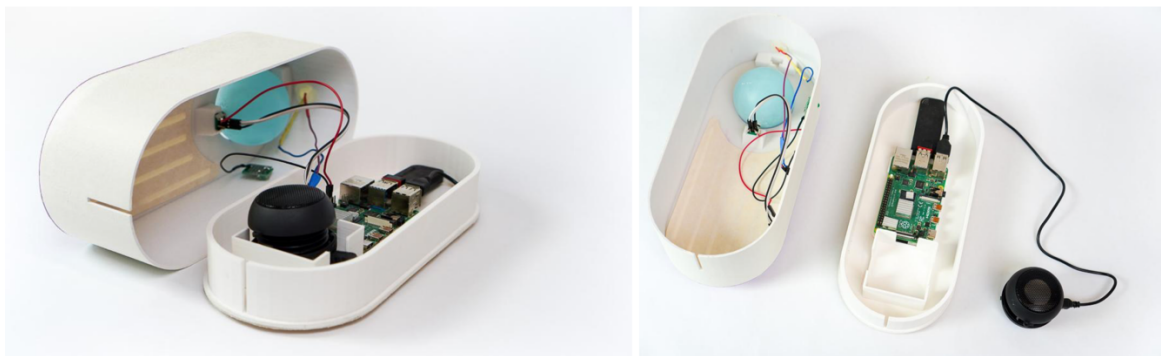
Figure 4: Broadcast is comprised of a Raspberry Pi microcontroller, a small speaker, and a 20-pin rotary encoder attached to the blue resin sphere.
